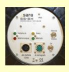
The SSDH sensors is extremely practical with its electric simple action switch for locking and unlocking the sensor to the borehole wall.
