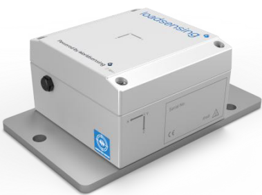
Fig. 1: Versatile horizontal surface mounting plate (LS-ACC-IN15-HP), recommended for both horizontal and vertical mounting. The plate has three clearance holes for MB anchor rods and an MB threaded hole available for installing a monitoring prism or a button head screw for precise leveling.
