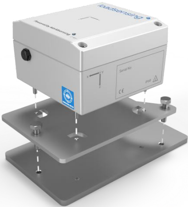
Fig. 2: Vibration Meter mounted on a double plate for horizontal surface mounting (LS-ACC-IN15DP). This is suitable for applications that need avoid opening the casing during installation.
