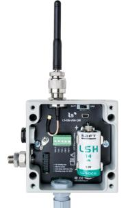
Fig. 1: An inner view of a vibrating wire data logger 1 channel. The data loggers are autonomous battery-powered devices with C-size batteries that can last several years with minimal to zero maintenance required
