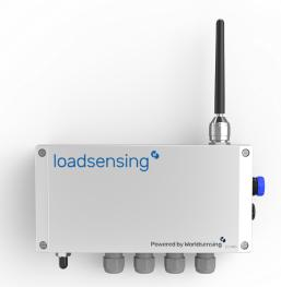
In terms of energy consumption. Worldsensing data loggers are autonomous battery-powered devices with C-size batteries that can last up to 10 years with minimal to zero maintenance required. The analog data logger is IP68 certified and tested from -40 °C to +80 °C.
